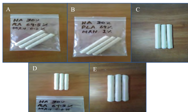
Figure 3: HA/PLA/MAH Biocomposites A) HA30/PLA/0.5MAH; B) HA30/PLA/1MAH; C) HA30/PLA/2MAH; D) HA30/PLA/4MAH; E) HA30/PLA/8MAH
