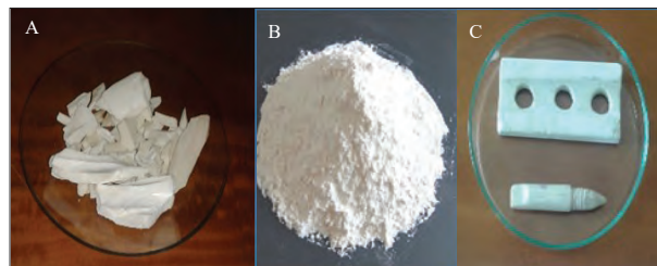
Figure 1: Hydroxyapatite A) Raw bone pieces; B) Bone hydroxyapatite; C) Trial bone plate
